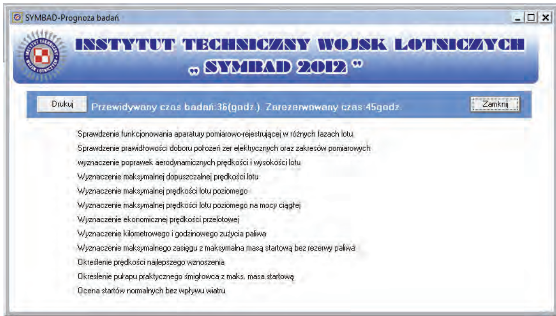
Fig. 2. A module to predict time needed for flight tests
