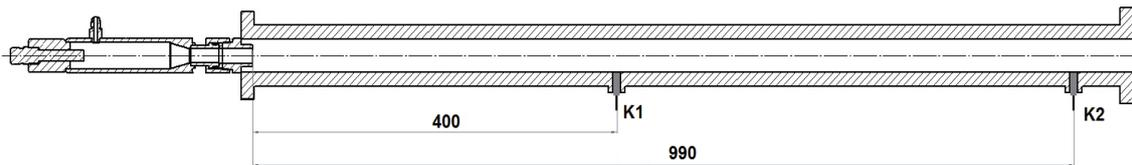
Fig. 4. The test stand scheme with measuring sensors (K1, K2) mounted
