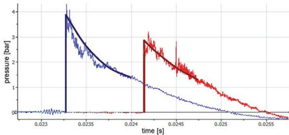
Fig. 8. Pressure Initiator – pressure 1 bar (test no. 32)
