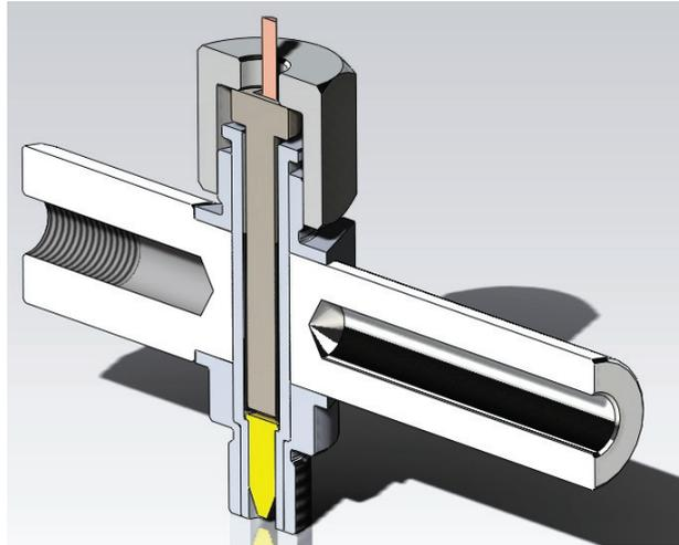
Fig. 3. Blank Ammunition Initiator
