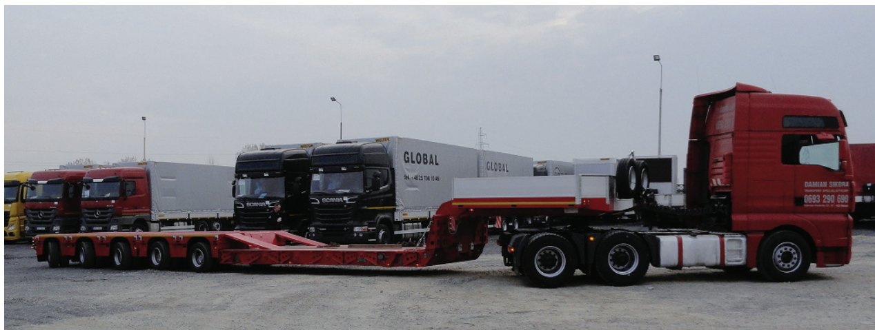
Fig. 9. Prototype of the semi-trailer coupled to a three-axle tractor unit
