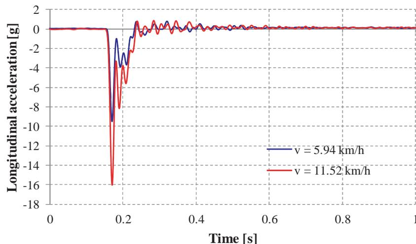
*Fig. 3. Comparison of the longitudinal acceleration for the trial 3 and 4*
