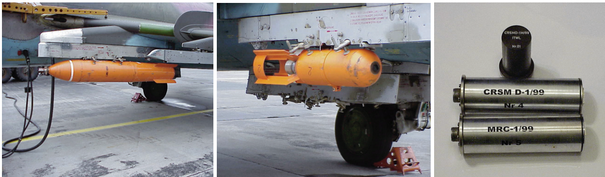
Fig. 3. Data recorders for flight parameters installed on avionic bombs with standard weight of 250 and 50 kg
