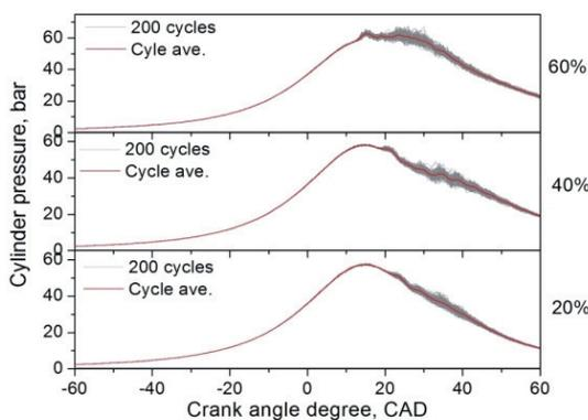
Fig. 2. Cylinder pressure for B100 at three different engine loads; 20%, 40% and 60%
