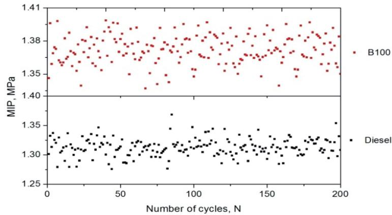
Fig. 6. MIP for mineral diesel and B100 at an engine load of 40% with a constant engine speed of 2500 rpm
