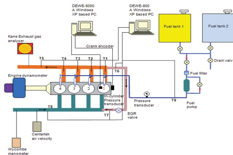
*Fig. 1. Schematic diagram of a Mitsubishi 4D68 diesel engine system*
