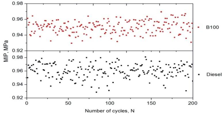
Fig. 5. MIP for mineral diesel and B100 at an engine load of 20% with a constant engine speed of 2500 rpm
