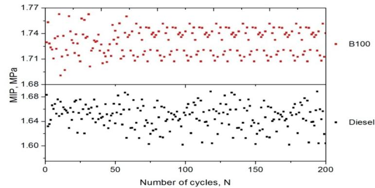
Fig. 7. MIP for mineral diesel and B100 at an engine load of 60% with a constant engine speed of 2500 rpm
