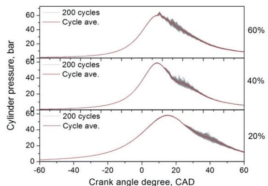
Fig. 3. Cylinder pressure for mineral diesel at three different engine loads; 20%, 40% and 60%
