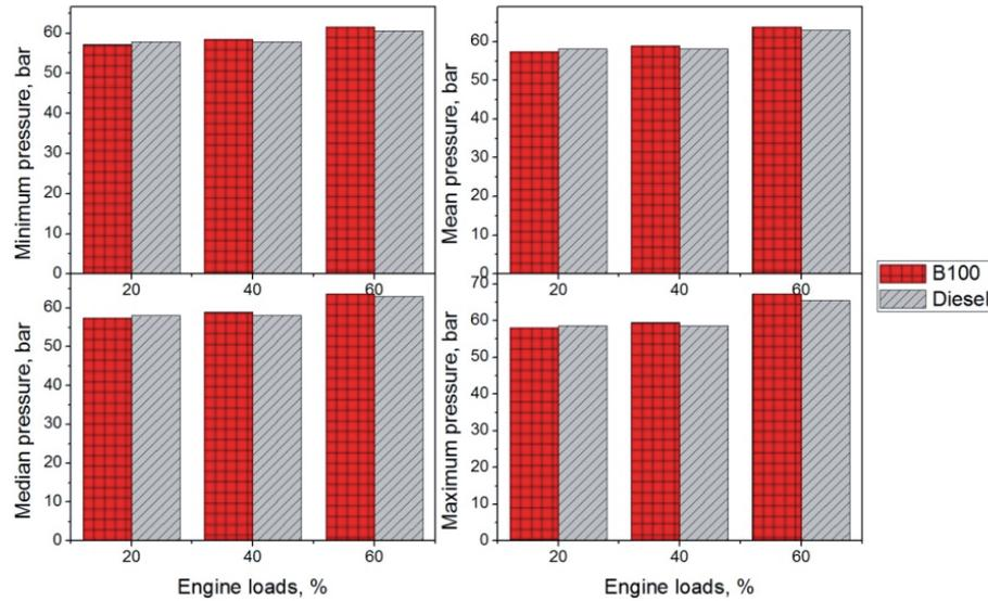
Fig. 4. Cylinder pressure statistical analysis for B100 and mineral diesel at three different engine loads; 20%, 40% and 60%
