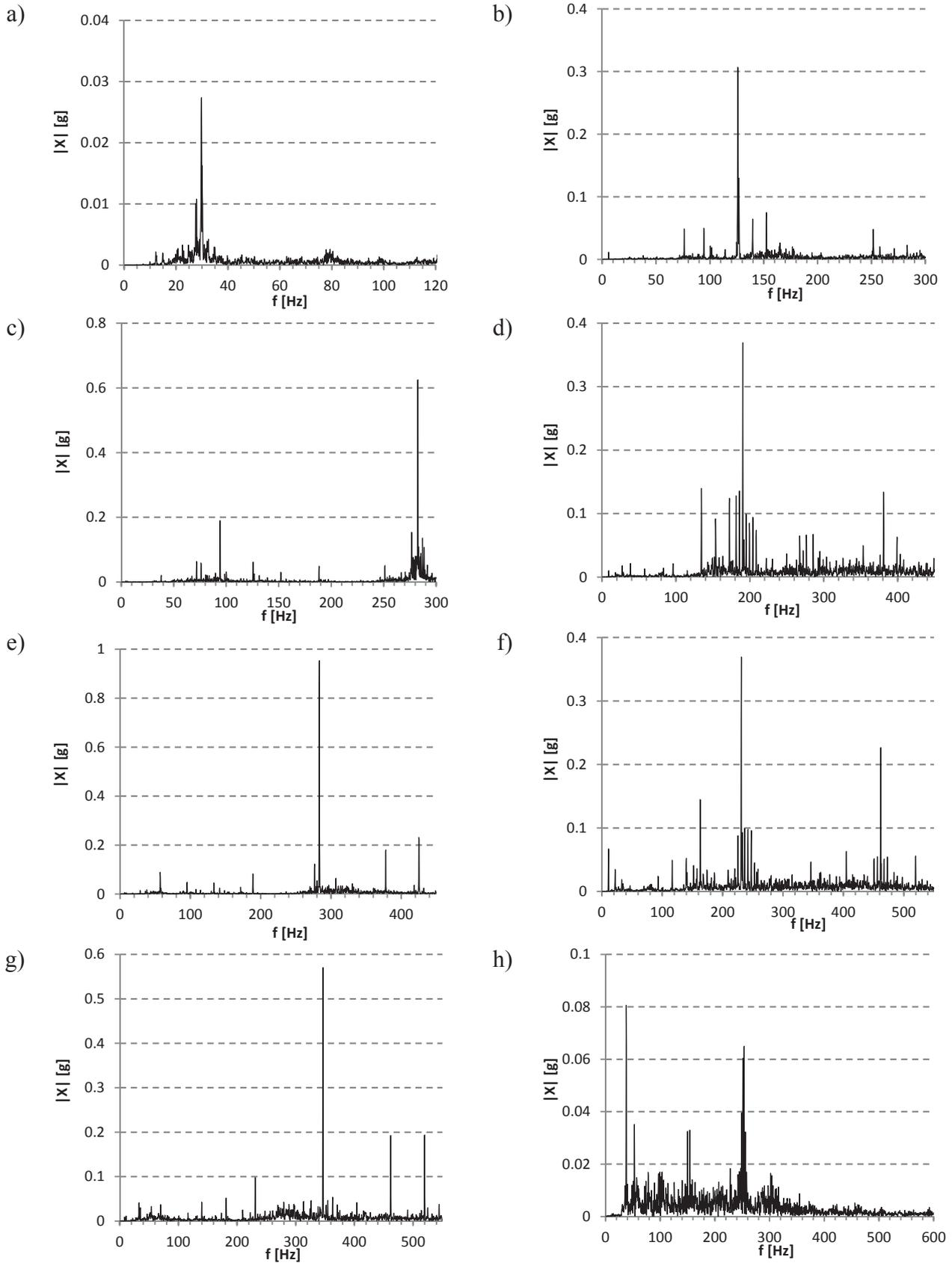
Fig. 6. Sample spectra of vibration signals recorded during the tests: a) the internal gear, measuring point 1,  $n_{bja1}$ , b) internal gear, measuring point 2,  $n_{Mo}$ , c) the gear extreme, measuring point 5,  $n_{Mo}$ , d) the internal gear, measuring point 1,  $n_{Mo-Ne}$ , e) extreme gear, measuring point 5,  $n_{Mo-Ne}$ , f) the internal gear, measuring point 1,  $n_{Ne}$ , g) on the gear extreme, measuring point 5,  $n_{Ne}$ , h) on the gear measuring point 5,  $n_{max}$
