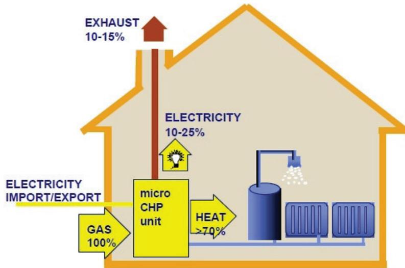
Fig. 3. Principle of operation of CHP systems
