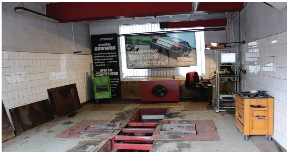
Fig. 1 VT-2 chassis dynamometer at V-tronic company
