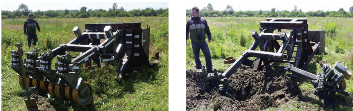
Fig. 6. Mine flail after detonation
