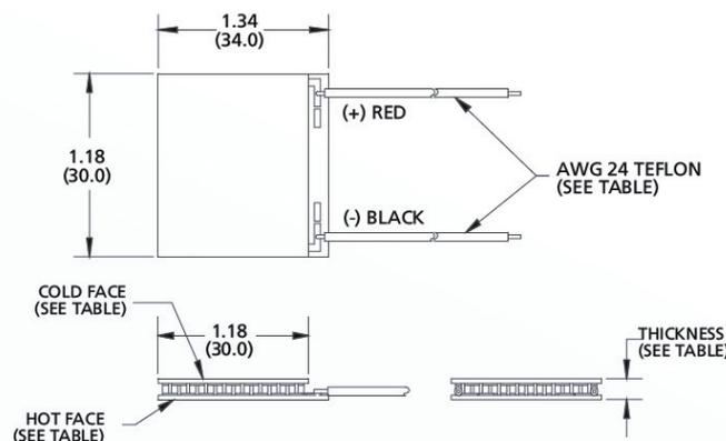
Fig. 1 Dimensions of Peltier module HT4, 12 [10]
