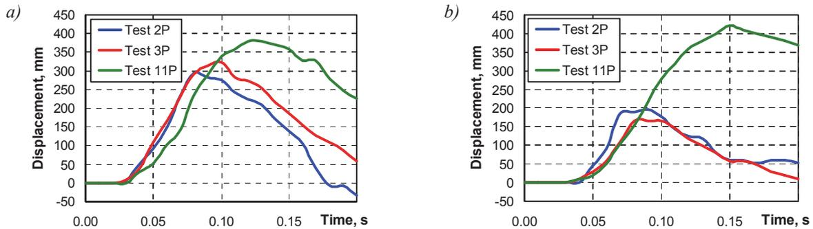
Fig. 9. Longitudinal shoulder (a) and hip displacement (b)
