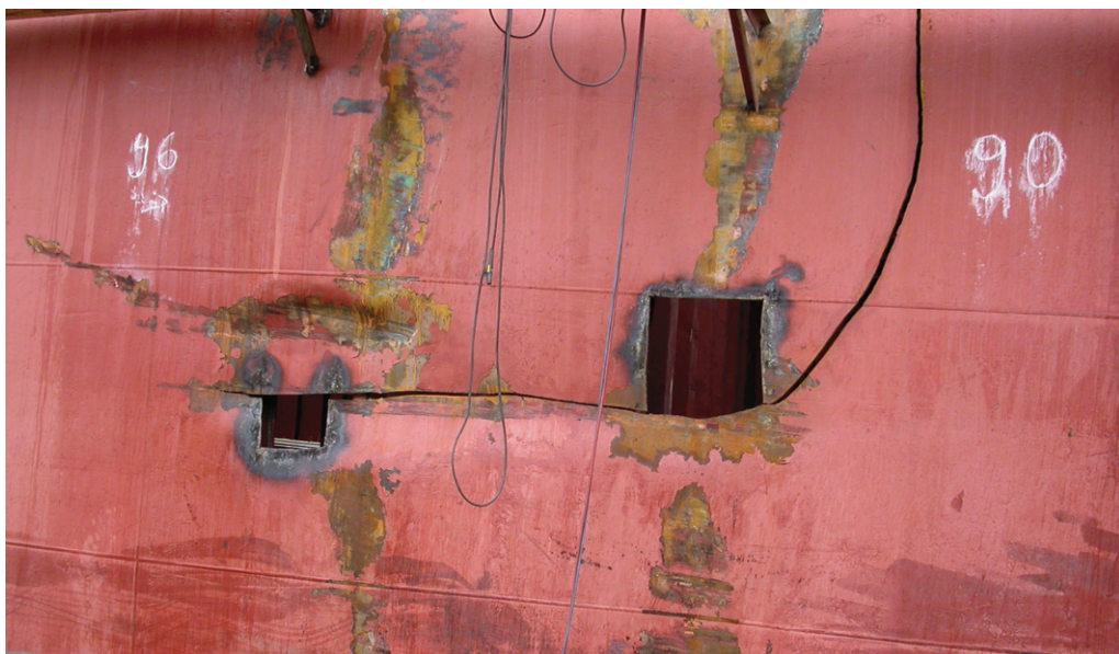
Fig. 4. Repair the ship after damage to the hull in a collision
