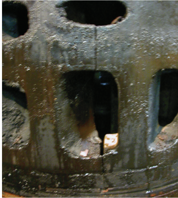
Fig. 5. View of cracked cylinder liner
