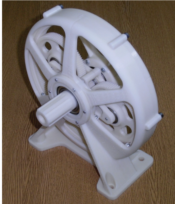
Fig. 2. A model of planetary gearing made by FDM method
