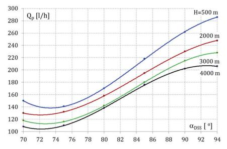
Fig. 7. Fuel consumption of the TWD-10B/PZL-10S engine as a function of variable flight altitude
