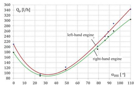
Fig. 4. Fuel consumption of TWD-10B/PZL-10S engines as a function of the tilt angle  $\alpha_{DSS}$  for the Engine Control Lever (DSS)
