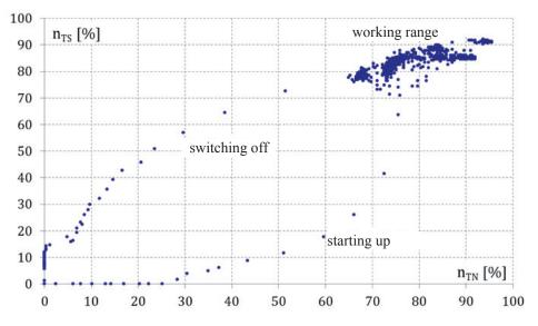
Fig. 3. Interaction between the turbocompressor and the driving turbine of the TWD-10B/PZL-10S engine
