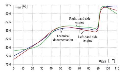
*Fig. 2. Relationships between driving turbine rpm for the right-hand side and left-hand side engines and the tilt angle of the Engine Control Lever (DSS)*
