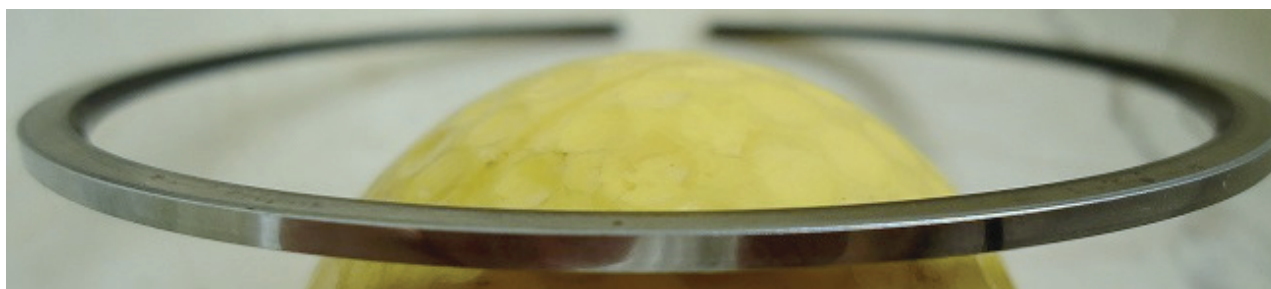
Fig. 2. View of side surface of the first ring of the cylinder No. 1
