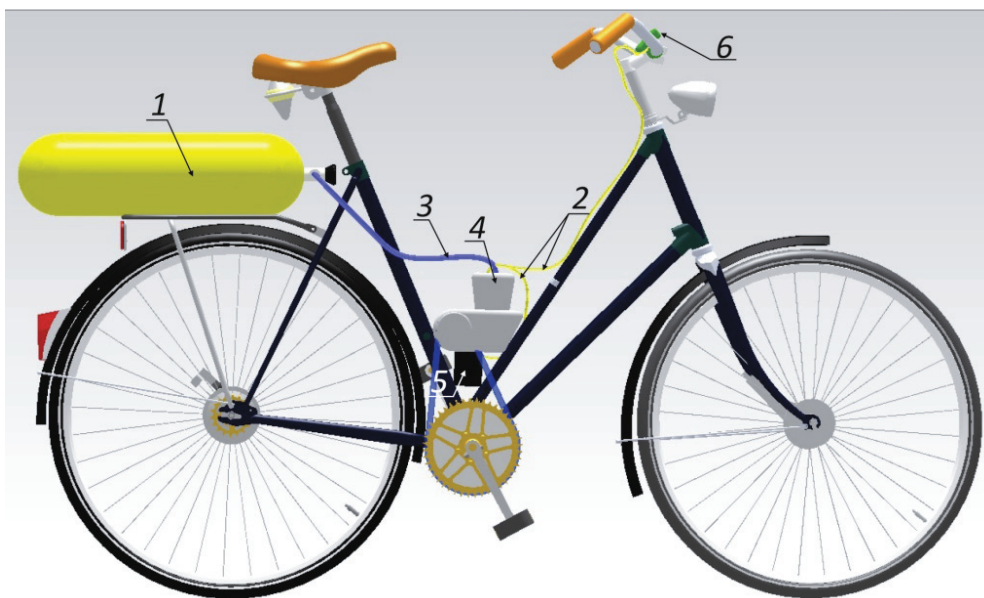
Fig. 2. Visualization of conception of bike with two presser pneumatic propulsion 1 – high-pressure tank, 2 – pneumatic connections, 3 – pneumatic engine, 4 – battery, 5 – electrical wiring, 6 – microcontroller
