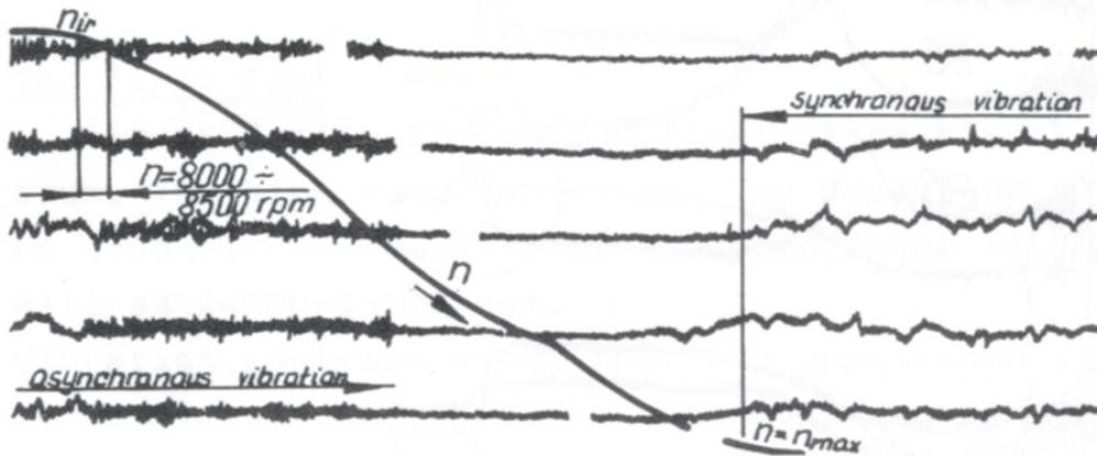
Fig. 1. Typical representation of the first stage compressor blades vibration during engine acceleration
