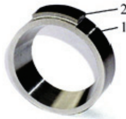
Fig. 1. The sliding pair: 1 – ring specimen, 2 – counterpart
