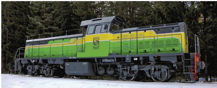
Fig. 3. The TEM9H Sinara Hybrid shunting locomotive [5]
