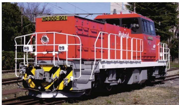
Fig. 1. Prototype of the Toshiba HD300 shunting locomotive [2]
