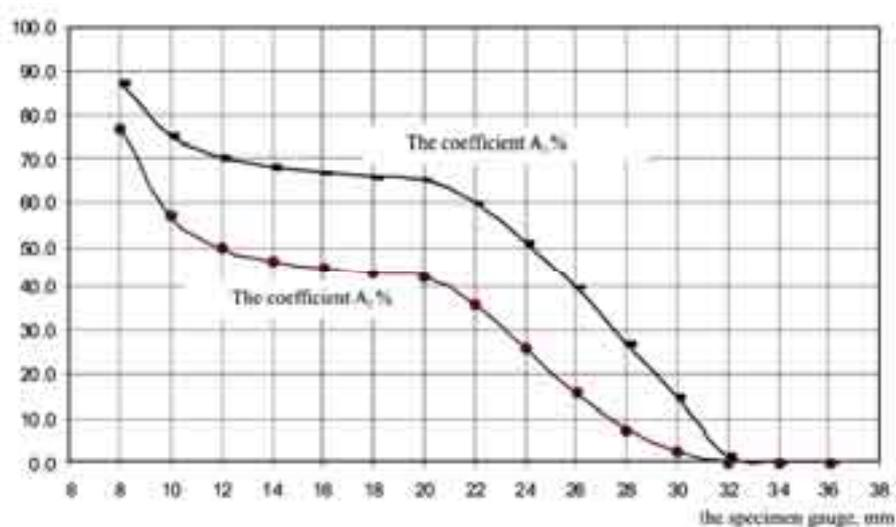
Fig. 8. The values of  $A_2$  and  $A_3$  for the 10GHMBA steel as a function of the specimen gauge
