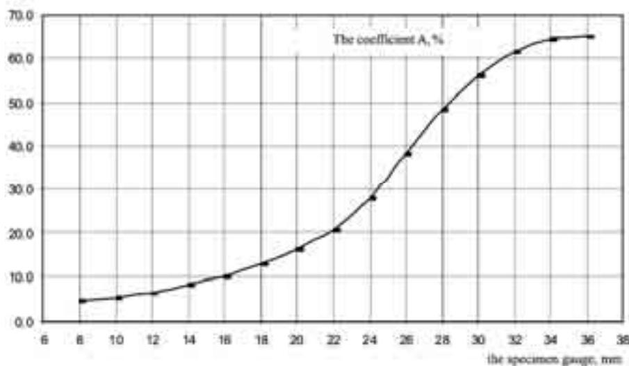
Fig. 7. The values of  $A_1$  for 10GHMBA steel as a function of the specimen gauge
