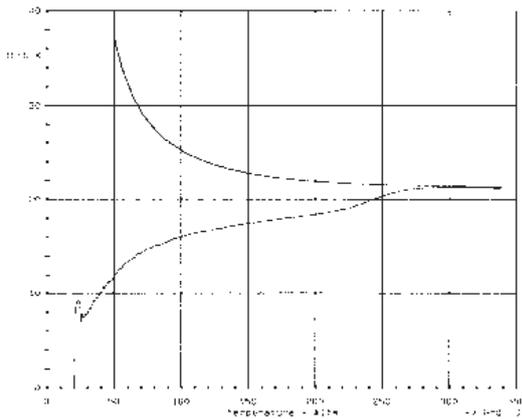
Fig. 3. The course linear coefficient  $\alpha$  thermal expansion  $\alpha$  in the function temperature (T) during heating and cooling of the standard overeutectic silumin of coefficient  $\alpha$  during the piston cooling equal to the coefficient  $\alpha$  within the range temperatures 340<sup>0</sup>C-300<sup>0</sup>C and higher below temperatures 300<sup>0</sup>C
