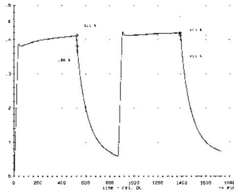
Fig. 16. The course of the relative extension in the function of time in the stabilization of the composite piston at the temperature 225<sup>0</sup>C
