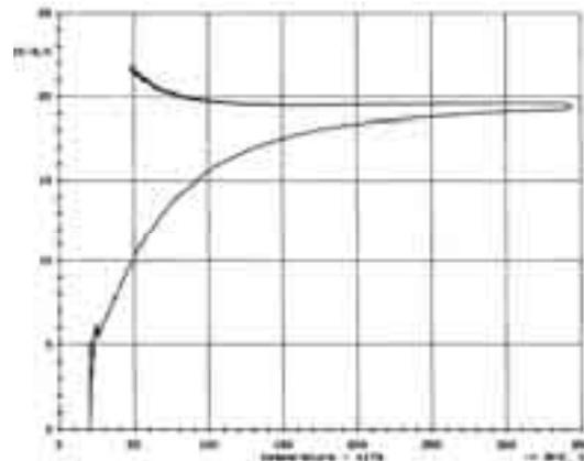
Fig. 4. The course of the linear coefficient  $\alpha$  of thermal expansion  $\alpha$  in the function of the temperature (T) during the heating and the cooling of the standard overeutectic silumin of greater coefficient  $\alpha$  during the piston cooling than the coefficient  $\alpha$  during heating
