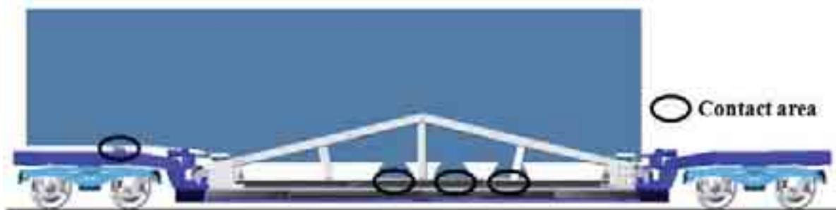
Fig. 6. Constraints mapping fixing of the semitrailer in the saddle and additional contact areas of semitrailer wheels with wagon model
