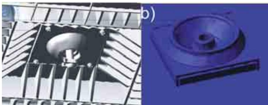
Fig. 4. Model of swivel pin used as central junction of floor rotation a) loading floor – down view, b) support – top view
