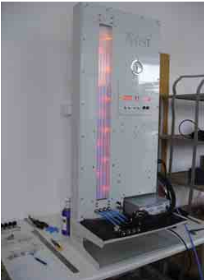
Fig. 1. Measuring device used to measure the flow rate of injectors
