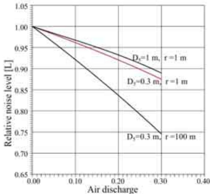
Fig. 5. Influence of air supply from behind the compressor to the place behind the turbine onto a relative noise level depending upon the diameter of the discharge nozzle  $D_3$  and the radius  $r$
