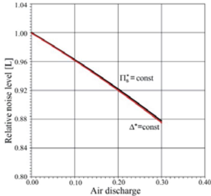
Fig. 4. Influence of air supply from behind the compressor to the place behind the turbine onto a relative level of engine noise depending upon the regulation method ( $D = 0.3 \text{ m}$ ,  $r = 1 \text{ m}$ )
