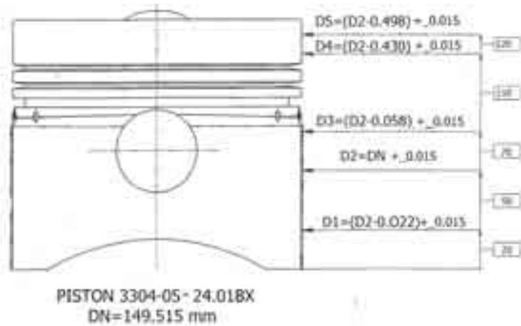
Fig. 1. Design of the 3304-05-24.01BX standard piston
