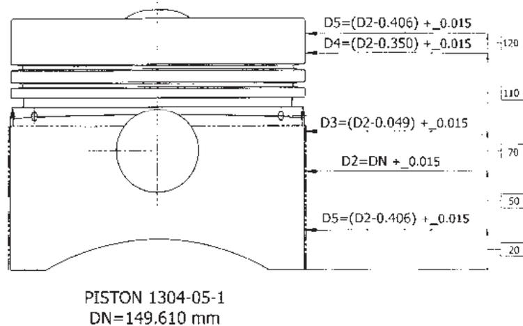
Fig. 3. Design of the 1304-05-1 novel piston
