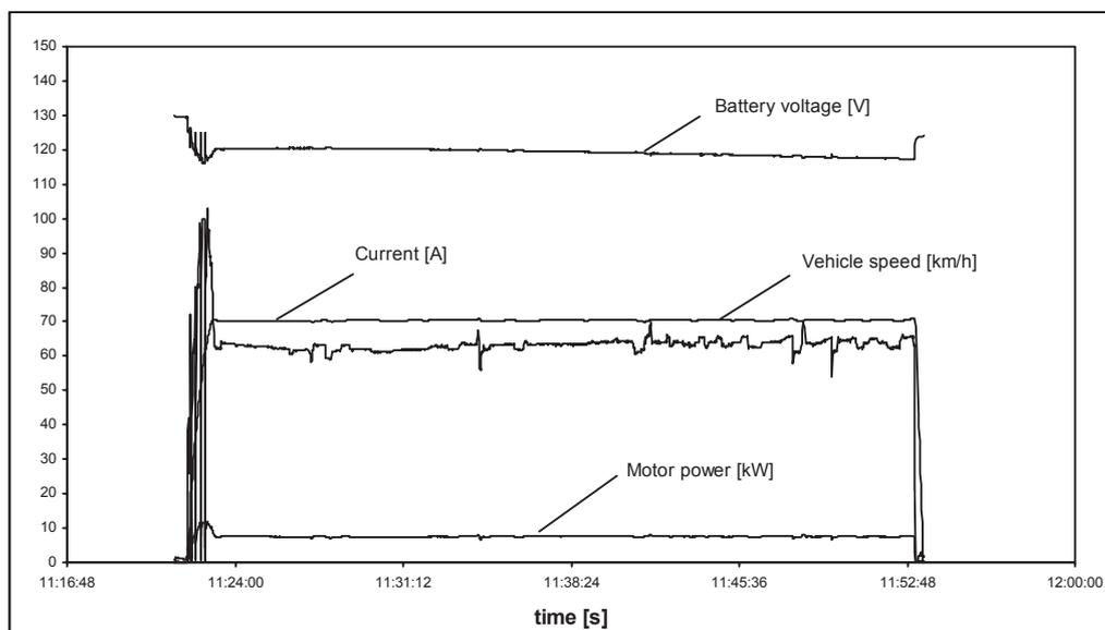
Fig. 5. The test at a speed of 70 km/h
