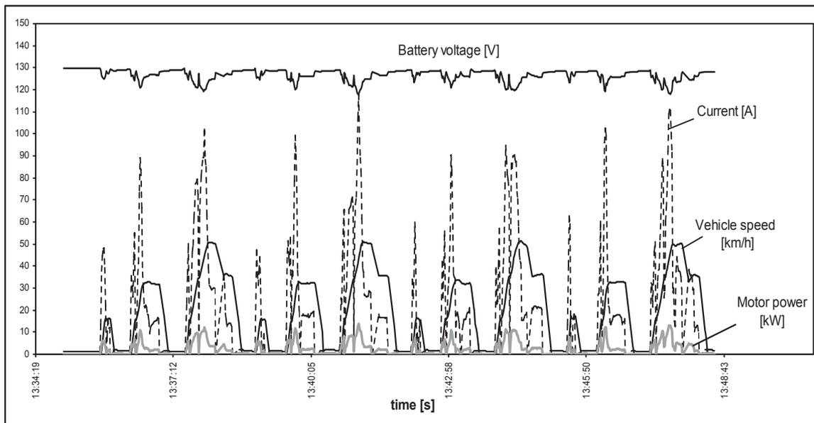
Fig. 11. The parameters of the selected NEDC test
