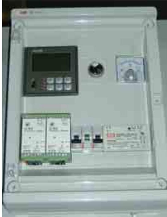
Fig. 2. Electrical power measuring and recording device
