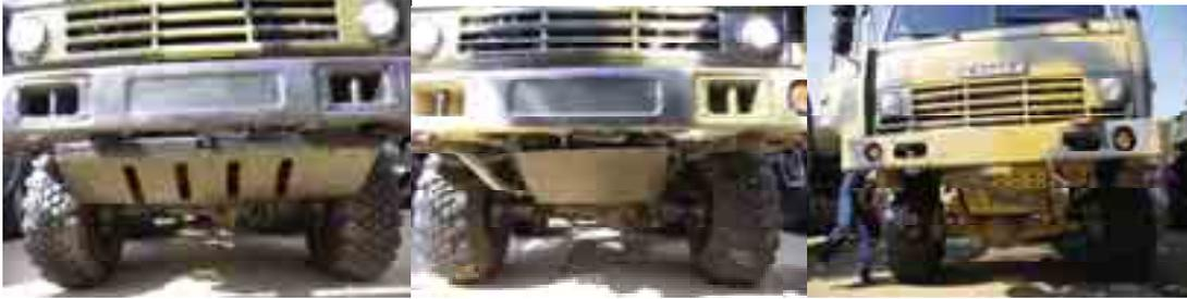
Fig. 11. Shields for driver's cabin in KAMAZ vehicle [www.bvt.narod.ru]
