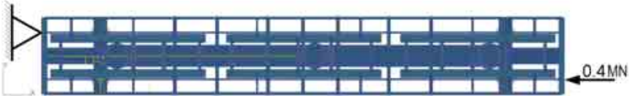
Fig. 7. Variant B: compression of the wagon with force of 0.4 MN applied diagonally on the level of buffers
