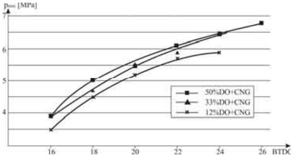
Fig. 3. The effects of advance angle of the pilot dose injection on the maximum pressure of combustion, at various proportions of diesel oil and CNG
