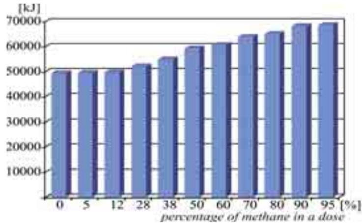
Fig. 4. Power demand of a dual-fuel self-ignition engine supplied with a mixture of methane and diesel oil
