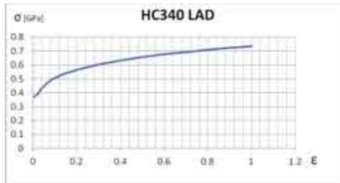
Fig. 4. Hardening curve for HC340 LAD g_0=2 mm
