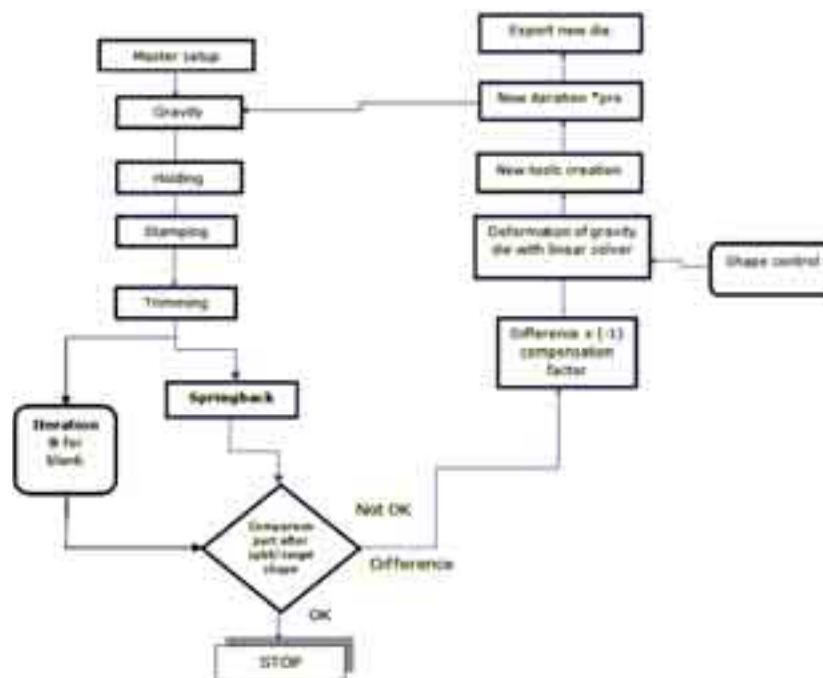
Fig. 2. Process of die compensation [9]
