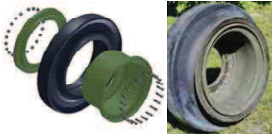
Fig. 1. Left - assembling diagram and Run Flat VFI 1400x20x10 G20, right - insert set mounted on the rim
