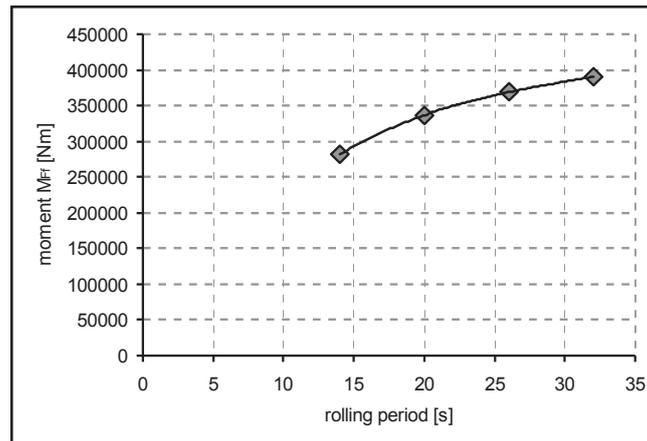
Fig. 11. Influence of ship's tank filling level on the free-floating component of the heeling moment due to liquid sloshing in the considered model tank
