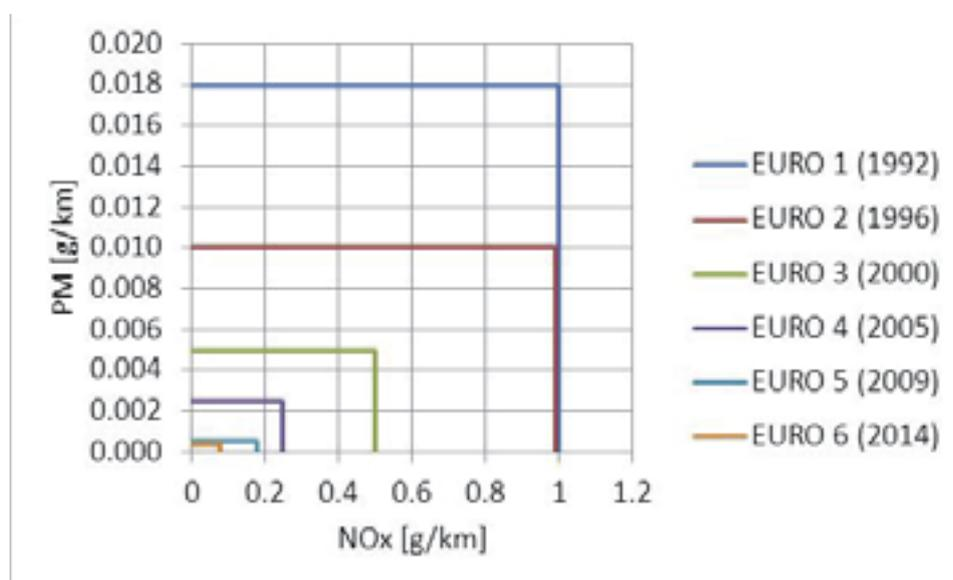
Fig. 1. EURO regulations in the area of NO<sub>x</sub> and PM emission
