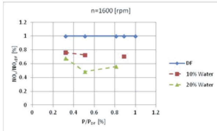
Fig. 5. Relative changes of value of the NO<sub>x</sub> concentration in exhaust gases of the engine in the function of relative load variations for different fuels, at the rotational speed of 1600 rpm
