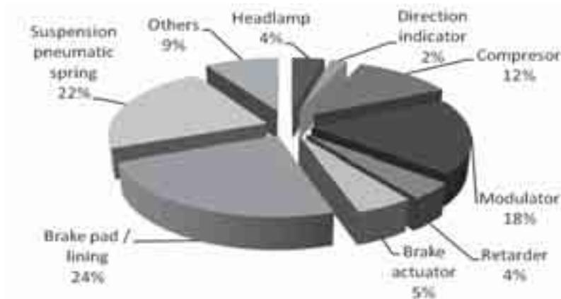
*Fig. 4. Structure of faults of particular parts for buses M3/III*
