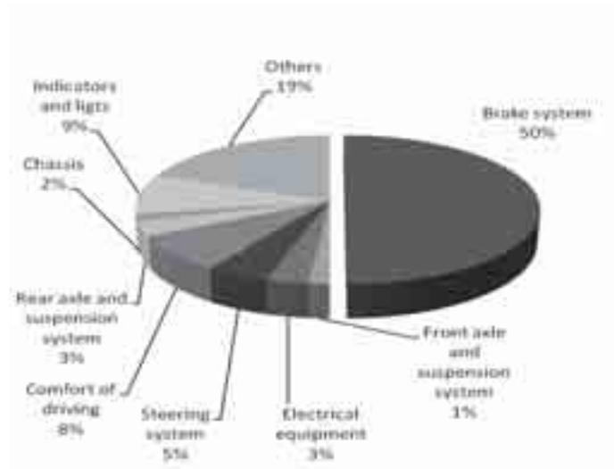
Fig. 2 Structure of vehicle faults
