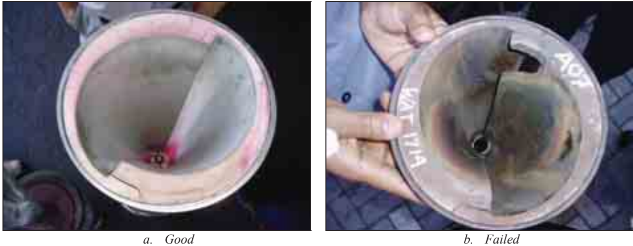
Fig. 2. Comparison between good and failed cone burners
