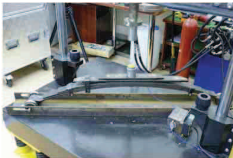
Fig. 3. Location of double spring on support plate of impact hammer
