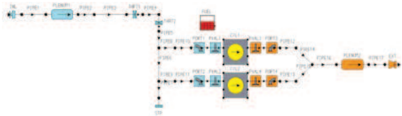
Fig. 3. Virtual model of the combustion engine Lombardini LGW 702, created with the program LES
