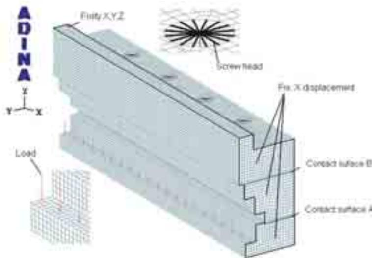
Fig. 5. Grid numerical model with boundary conditions
