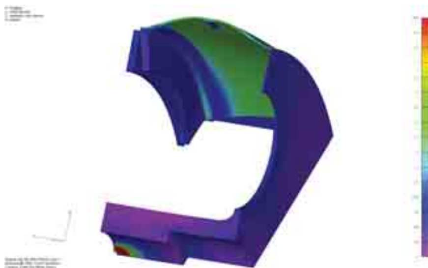
Fig. 5. Total displacement of nodes in computational model for 10000 [r / min]
