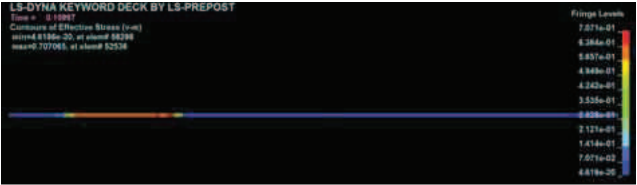
Fig. 8. Wave propagation through initial bar in t=0.15997ms
