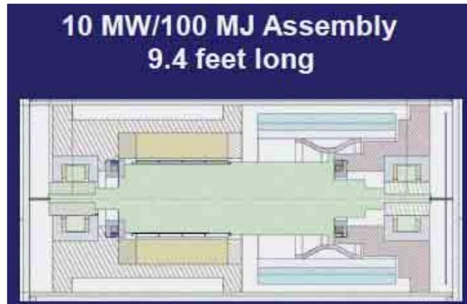
Fig. 9 Beacon POWER proposition of flywheel for naval ship of 10 MW (27.8 kWh) [8]
