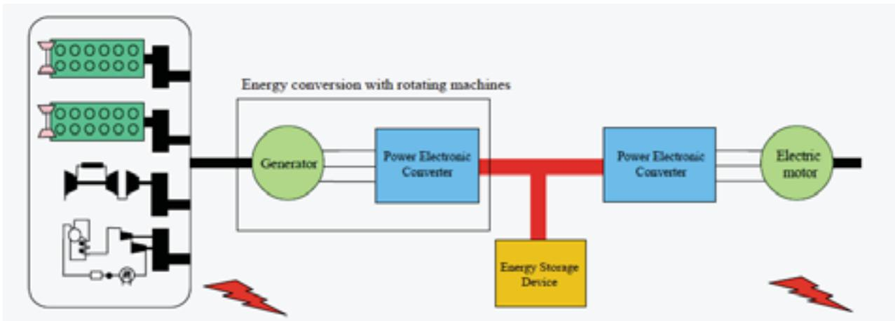
Fig. 1. Structure of combined ship's power plant [1]
