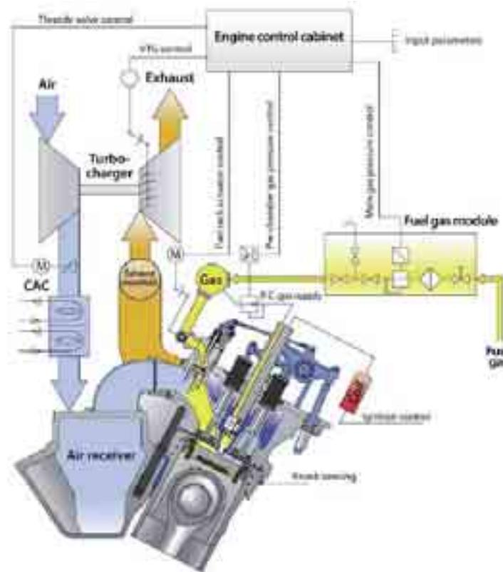
Fig. 3. Supplying fuel system of Bergen gas engine [1]
