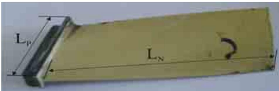
Fig. 1. I level compressor blades of the axial air turbine engine S0-3:  $L_N = 113$  mm,  $L_P = 40$  mm
