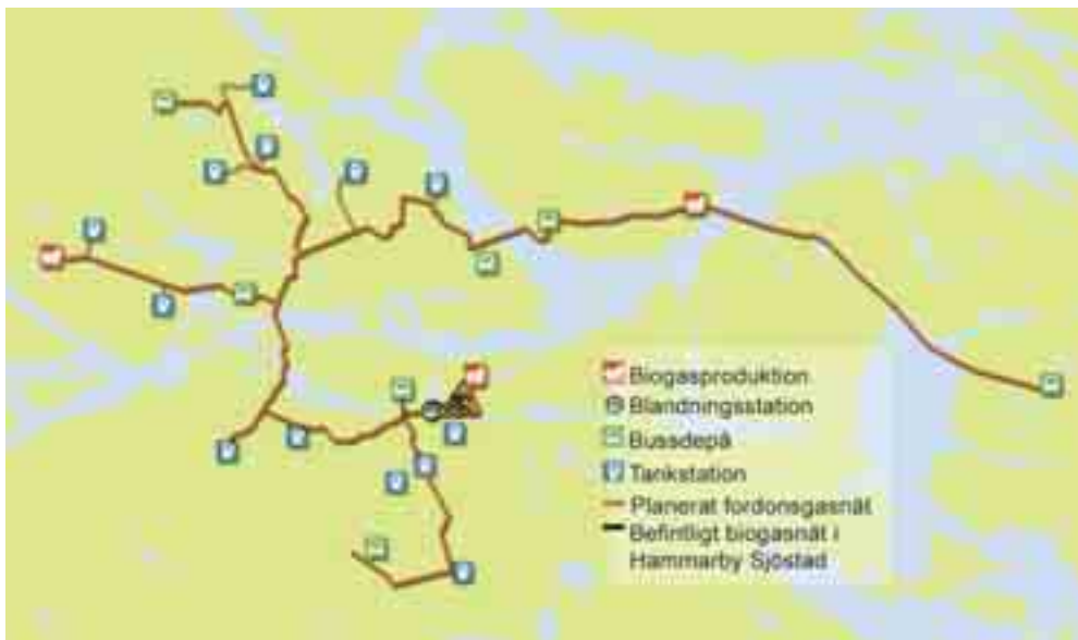
Fig. 1 Planned gas grid distribution of biogas in Stockholm [3]
