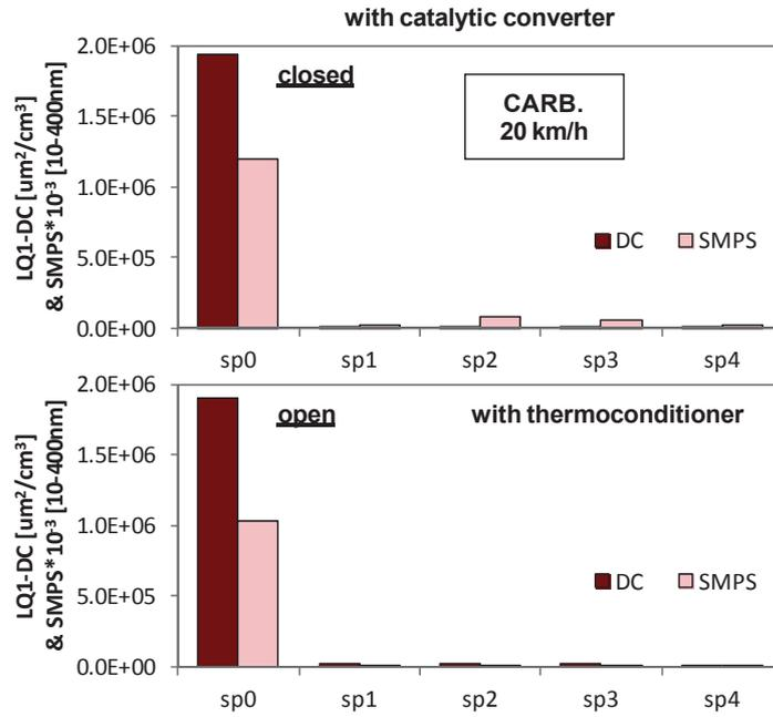
Fig. 11. DC signal & SMPS integral concentration from 10 to 400 nm at constant speed 20 km/h and different sampling points of the exhaust pipe and CVS tunnel with catalyst
