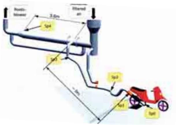
Fig. 3. Sampling positions (Sp) used in the tests
