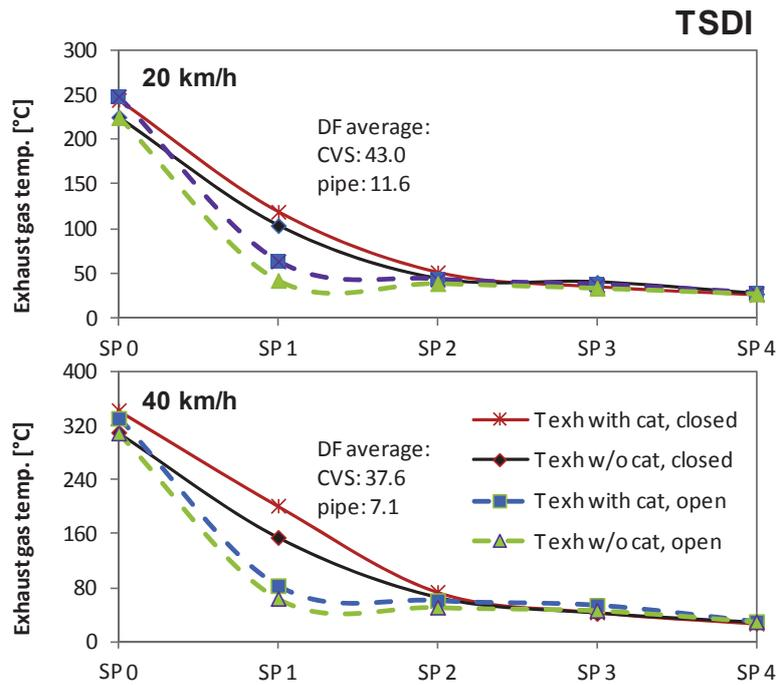
Fig. 5. Gas temperatures and dilution factors in the exhaust system at constant speeds 20 & 40 km/h, with TSDI
