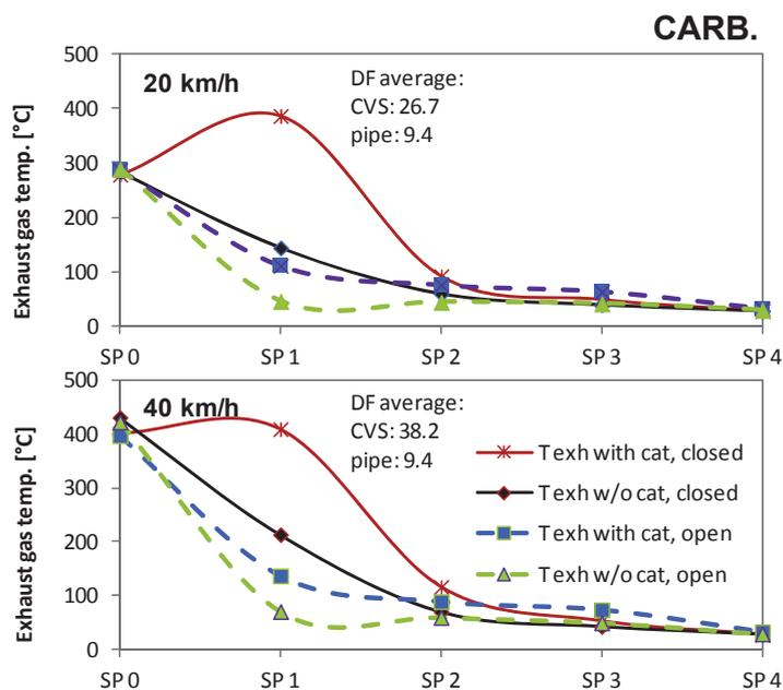
Fig. 9. Gas temperatures and dilution factors in the exhaust system at constant speeds 20 & 40 km/h, with Carb
