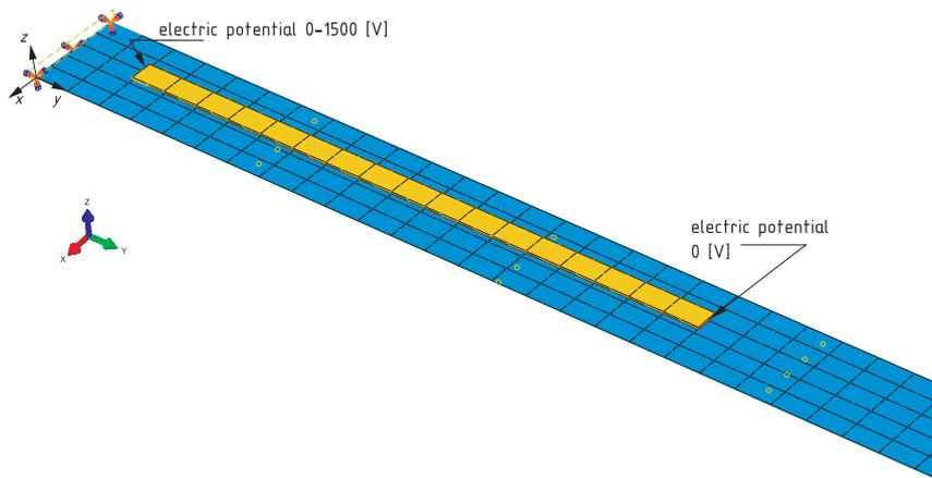
Fig. 5. Electric boundary conditions for the examined actuator
