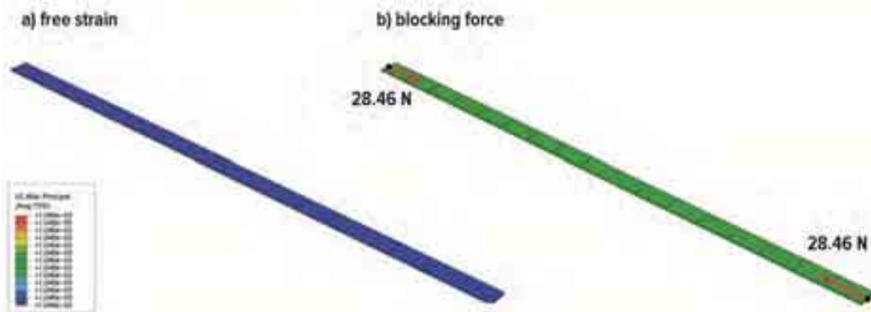
Fig. 2. Numerical tests for the separated M-8503-P1 piezoelement: a) free strain extension, b) blocking force
