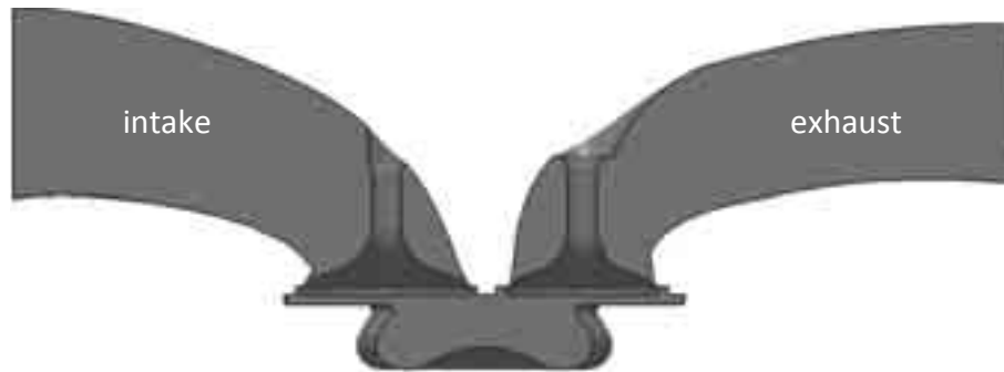
Fig. 2. Geometry in TDC of modelled test engine in CAD
