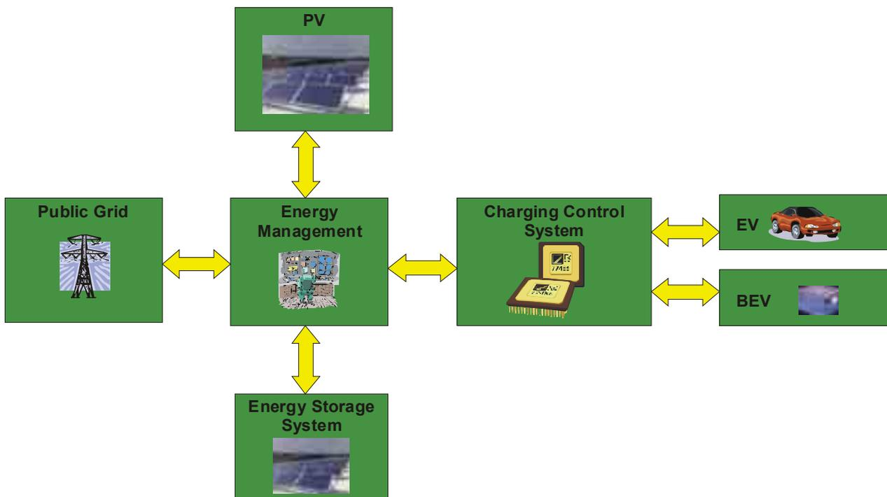
Fig. 1. Scheme of the charging station operation
