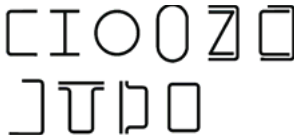
Fig. 2. Typical cross sections of profiles used in frames [5]
